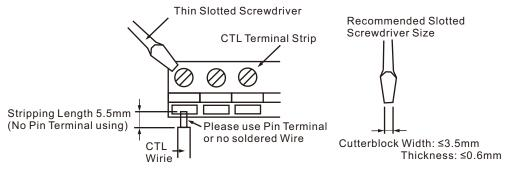
Fit CTL Wire into Terminal Strip
