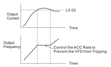
Fig. Stall Prevention Function During ACC (L3-01=1)
