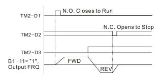
Fig. Terminal Signal Timing Sequence
