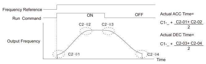
Fig. S-Curve Characteristic Timing Diagram
