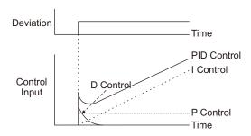
Fig. PID Operation
