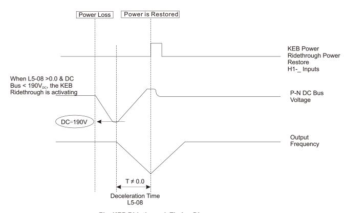
Fig. KEB Ridethrough Timing Diagram
