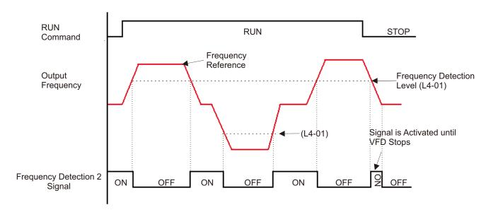
Fig. Frequency Detection 2 Timing Diagram
