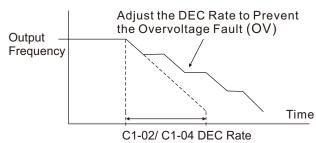
Fig. Stall Prevention Function During Deceleration (L3-04)
