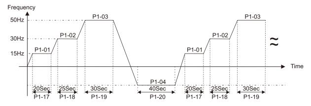
Fig. Continuously Executes Cycles Operation (P1-00= 2 or 5)
