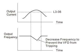
Fig. Stall Prevention Function During Running (L3-05= 1)
