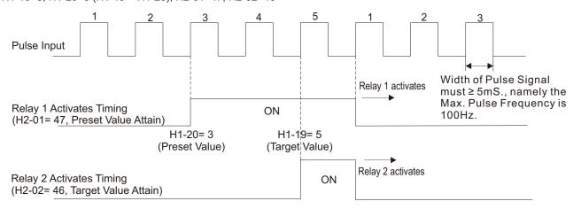
Fig. Counter Timing Diagram
