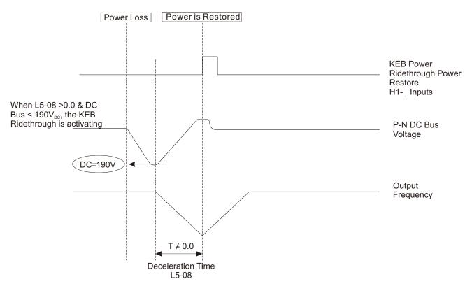
Fig. KEB Ridethrough Timing Diagram
